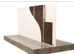
METAL STUD PARTITION WALL WITH INSULATION
