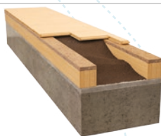
RESILIENCE ON NAILED HARDWOOD FLOOR OVER COCONUT FIBER
