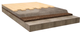
FLOATING SLAB WITH WOOD FLOORING
