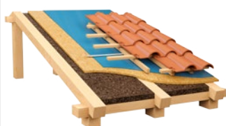
PITCHED ROOF WITH INTERNAL INSULATION BETWEEN RAFTERS
