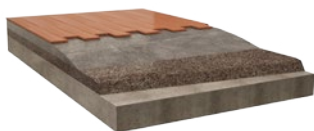
LIGHTWEIGHT CONCRETE - SCREED FILLING
