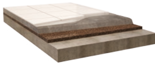
FLOATING SLAB WITH MOSAIC FLOORING
