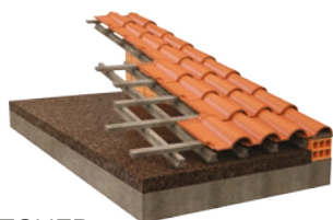
PITCHED ROOF WITH RIGID INSULATION OVER SLAB
