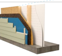
STANDARD LAP SIDING WITH EXTERIOR RIGID INSULATION
