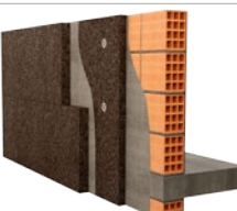
EXTERIOR CLADDING OVER INSULATION - CORK AT SIGHT
