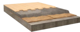
FLOATING SLAB WITH COCO FIBER
