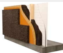
EXTERIOR CLADDING OVER WOODEN SUBSTRATE - CORK AT SIGHT
