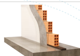
MASONRY WALL AND SLAB DISCONTINUITY
