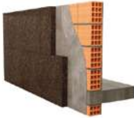
External walls Exterior cladding - cork at sight
