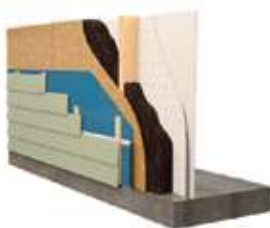
Interior solutions for exterior walls Internal insulation for external walls
