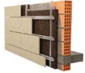
External walls Exterior cladding - cork at sight wave facade s1
