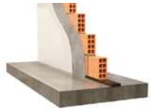
Internal partitions Masonry wall and slab discontinuity
