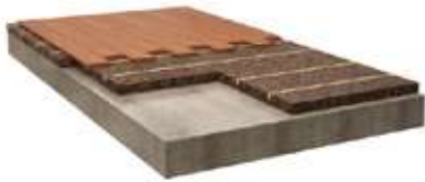
Slab and Floors Lightweight concrete - screed filling
