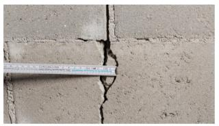
**3. Determine the crack width** AEROSANA VISCONN FIBRE bridges cracks of up to 20 mm (0.8") in width.
