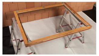
**1. Masonry or timber structure** CONTEGA SOLIDO SL-D is fitted before the window is installed. The frame is laid out flat with the interior side facing up.
