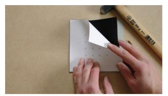
**1. Align the underlay, EPDM and template** Place the EPDM grommet on a cardboard underlay, put the template in place and align it.
