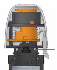
Splash-water protected due to mould seal
