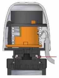
Splash-water protected due to mould seal
