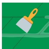
Sand the tile joints flush, fill any joints and sand again.
